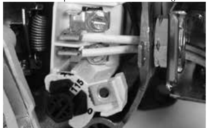
Figure 11: Voltage set to 115 volts, Dial Type
